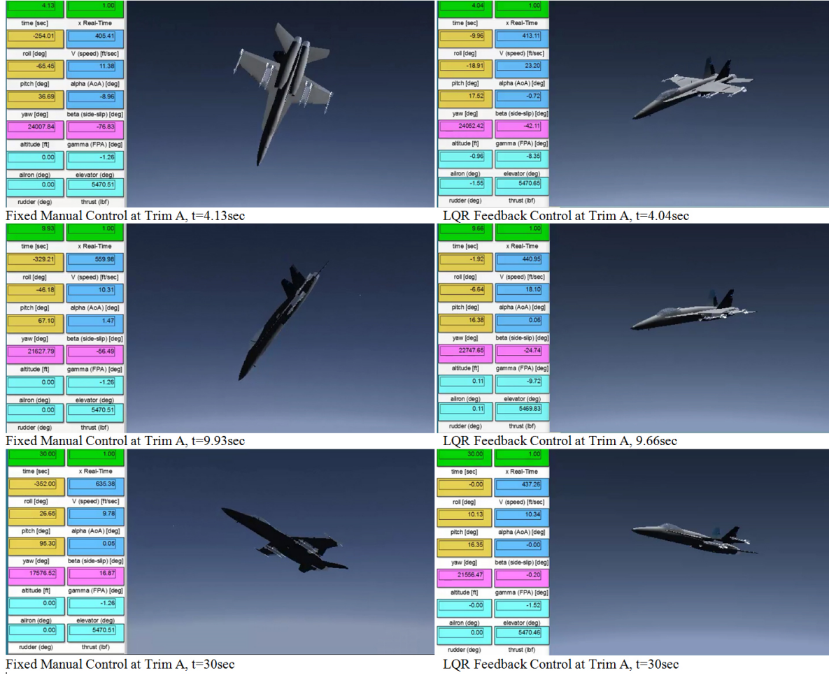
Figure 4. Snapshots of the aircraft flight with fixed manual control (left column) and with LQR feedback control (right column).
